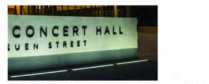
Ground directional lighting + lit letters shown above
